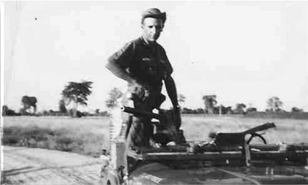
Photo of the author with the .30 cal. machine gun on the jeep in the Bomb Storage sector. Note the windshield tied down to permit the machine gun to swing 180 degrees.
